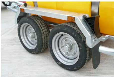
GALVANISED MUDGUARDS WITH SIDE REFLECTORS
