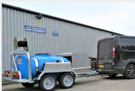
EASY-TOW DESIGN WITH FULL HIGHWAY APPROVAL AND INDESPENSION TWIN-AXLE RUNNING GEAR
