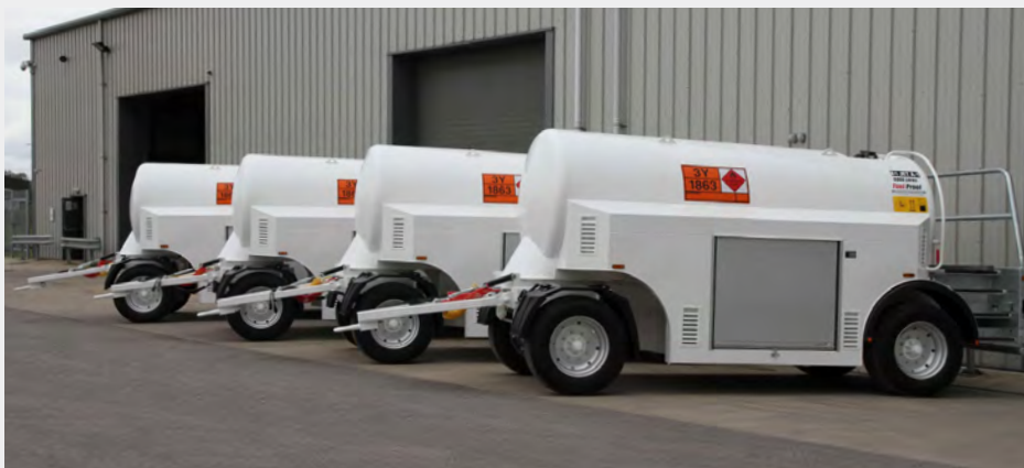
6000 LITRE ARTICULATED AVIATION FUEL BOWSERS SUPPLIED TO A NATIONAL AIR FORCE
