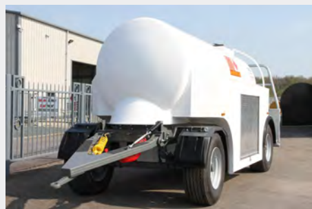
ARTICULATED ARRANGEMENT ON AIRFIELD TOW BOWSER
