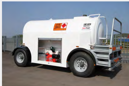
6000L AIRFIELD TOW BOWSER SHOWING CABINET OPEN FOR ACCESS TO FUEL DISPENSING EQUIPMENT
