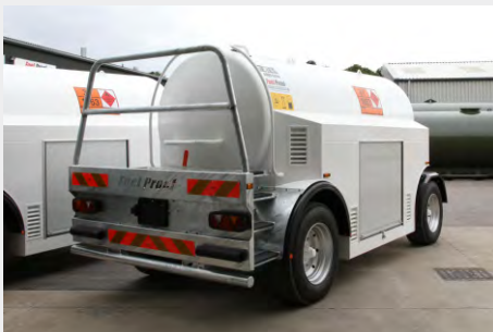
REAR ACCESS STEPS TO MANWAY/ INSPECTION HATCH
